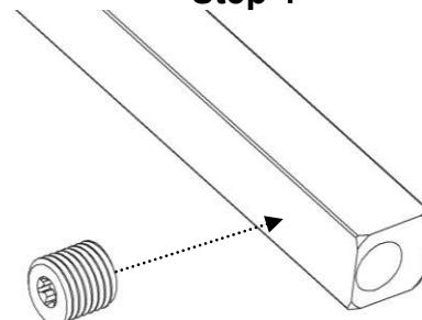
**Attention:** Insert the spindle in such a way that the point of the grub screw can break through the thinnest side.
